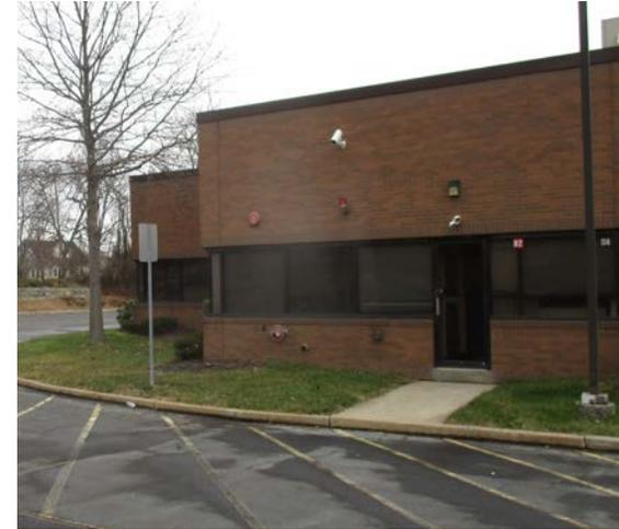
Sections of parking spaces can be converted to porous pavement to capture and infiltrate stormwater runoff from the parking lot. A preliminary soil assessment suggests that the soils have suitable drainage characteristics for green infrastructure.
