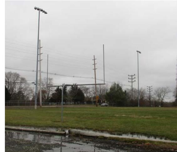
Rain gardens can be installed around the football field to capture, treat, and infiltrate stormwater runoff from the parking lot and roadway. A preliminary soil assessment suggests that more soil testing would be required before determining the soil's suitability for green infrastructure.
